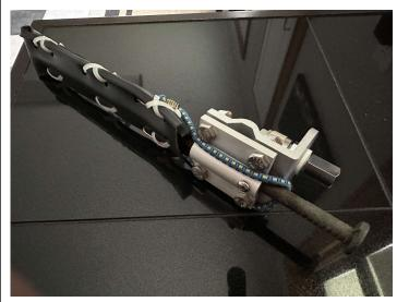
This is used to support a collapsible 17' whip for a ground mount vertical, but it also fits into the PEX on the stay of the PERformer support tube. The top of the spike is used to hold the guy loops.
